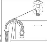
**Directly into a drain pipe at a height** of not less than 60 cm and not more than 90 cm.
